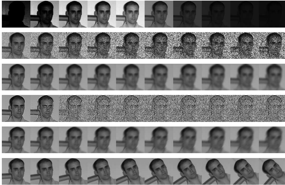
Fig. 2. The six test. From top to bottom: lighting, speckle, blurred, unsharp, motion, rotation.
