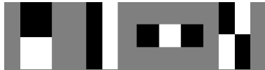
Fig. 3. Sample filters from the Viola-like filter bank. From left to right: horizontal and vertical edge detectors, vertical bar detector and special diagonal detector.
