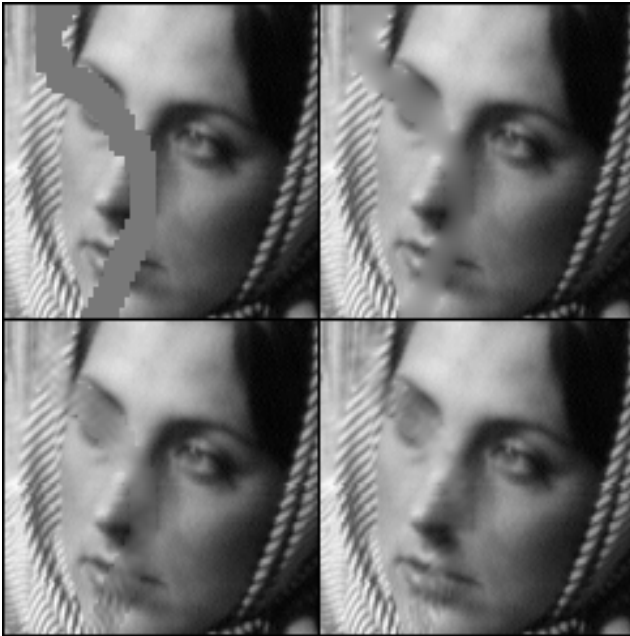
Fig. 2. Top-left , 120 \times 120 cropped degraded Barbara (24.19 dB). Top-right , Fast-inpainting (32.71 dB). Bottom - left , EM-inpainting (Curvelets + Local-DCT, 34.14 dB). Bottom-right , \ell_0 -GM (6-scales Curvelets, 34.92 dB).
