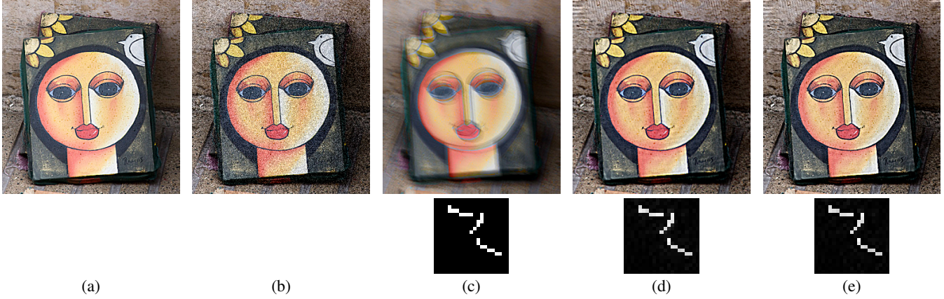
Figure 1: (a) original image, (b) observed noisy image simulating a short-exposure acquisition, (c) blurred image simulating long-exposure photographs. The blur used to generate this image is shown below the image. (d) using the method in [2], and (e) Estimated image and its corresponding blur using the proposed method with \lambda_1 = 0.5 .
